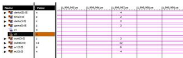
Fig 7. Output Waveform of proposed GF multiplier
