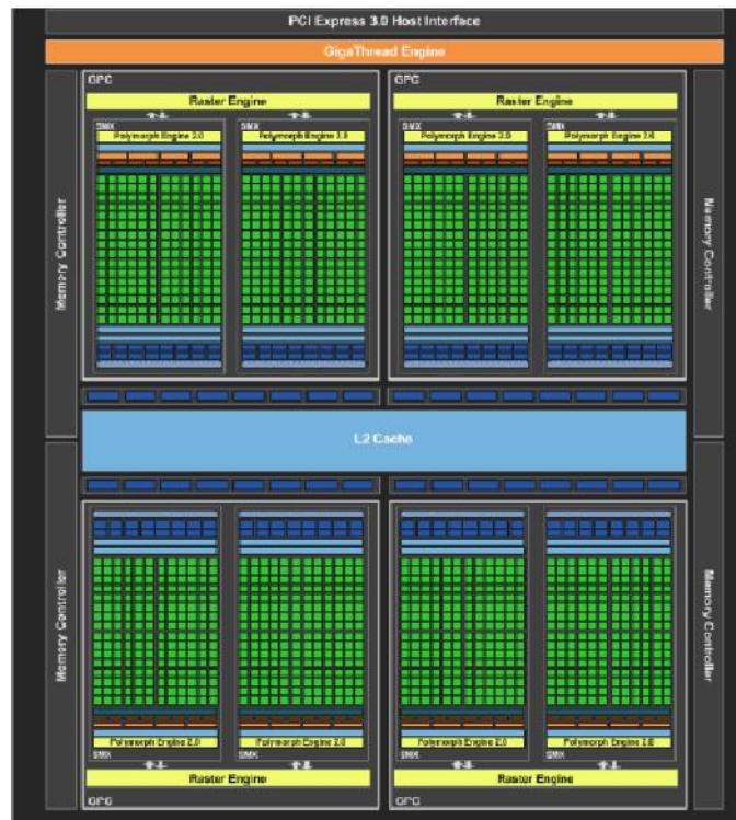
Fig 1: GTX 680 Architecture Block Diagram [10]
