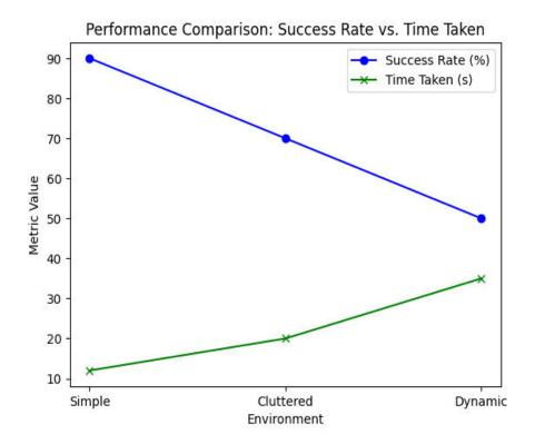
The graph demonstrates a trade-off between success rate and time efficiency. As the complexity of the environment increases, both the success rate decreases and the time taken increases. This indicates that the robot's performance is highly dependent on the environment's complexity.
