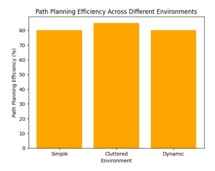
Path planning efficiency is slightly affected by dynamic obstacles and cluttered environments. However, the overall efficiency remains high, especially in more controlled environments, suggesting that the A\* path planning algorithm is effective in navigating these scenarios.
