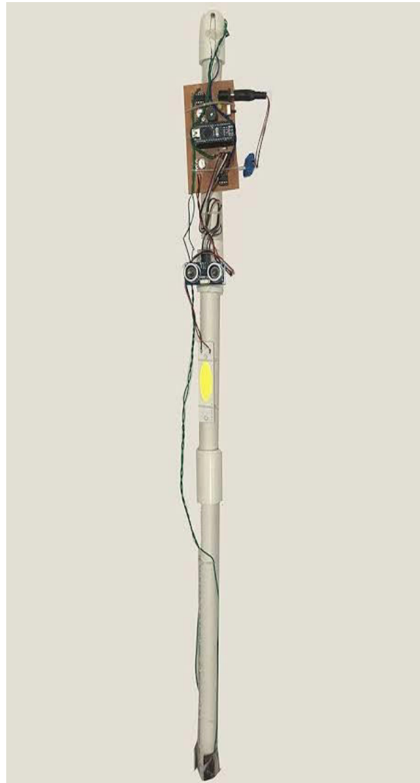
Fig 3: Implementation of Haptic navigator stick
