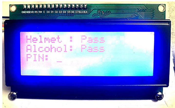
Fig 5.4: When both the helmet and alcohol detection systems register a pass state and ignition button is pressed, the system requests for a PIN to initiate the ignition process
