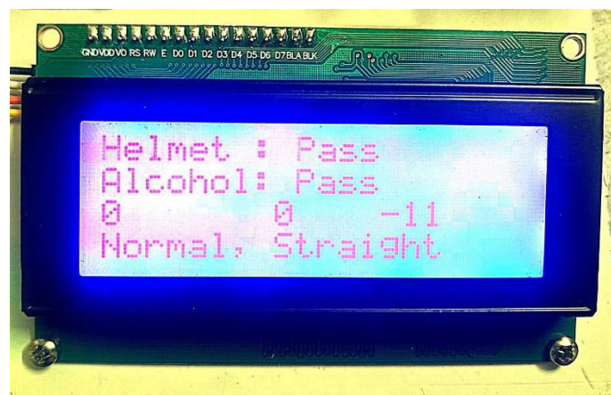
Fig 5.6: The Gyroscope constantly measure the tilt angle of the system and is displayed on the LCD screen.
