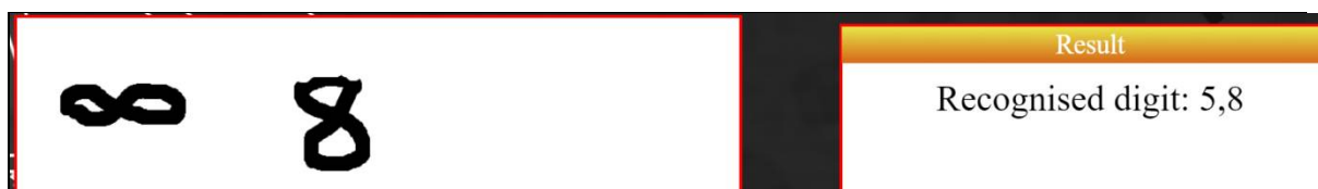
Picture 4.1: Wrong recognition because of orientation of 8
