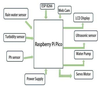
The dam control system is designed with the integration of multiple subsystems that work together to monitor and manage dam operations. The major subsystems involved are crack detection, water level detection, rain sensing, and
