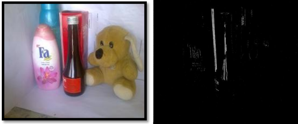
(a) (b) Fig.3 (a) Image taken from 2MP mobile (b) Result of new proposed canny operator.
