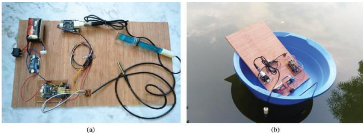
Figure 10: IoT based monitoring system: (a) Shows the device, which shows the connecting equipment and (b) is the real-life experiment of the device in which the device is measuring the water of a pond
