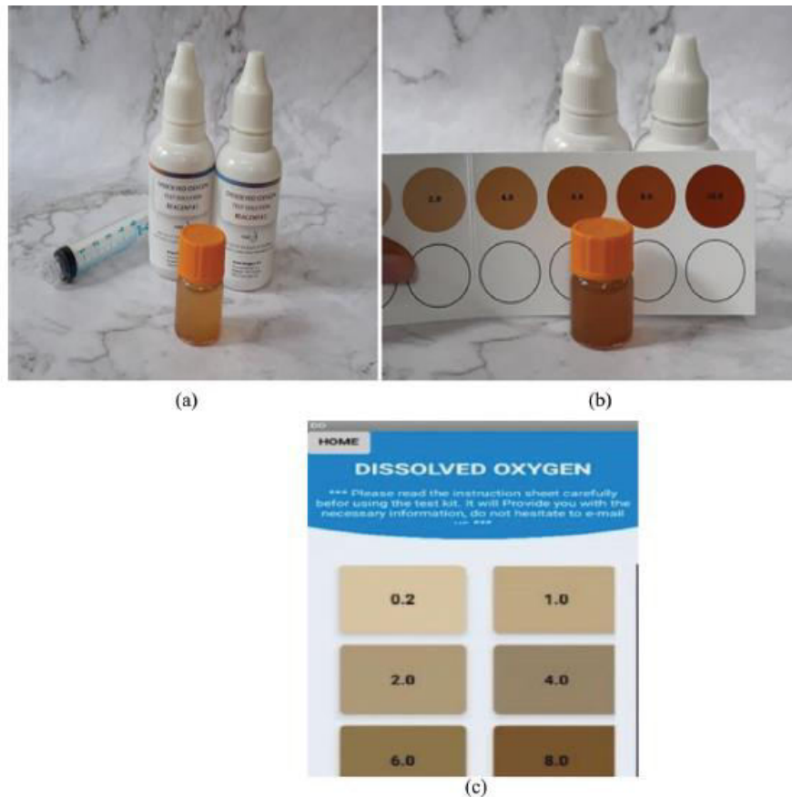
Figure 14: Result of dissolved oxygen (a) is the solution made by the Kit, (b) is the solution with the matching with the provided color code and (c) Shows the interface of the application of the color code
