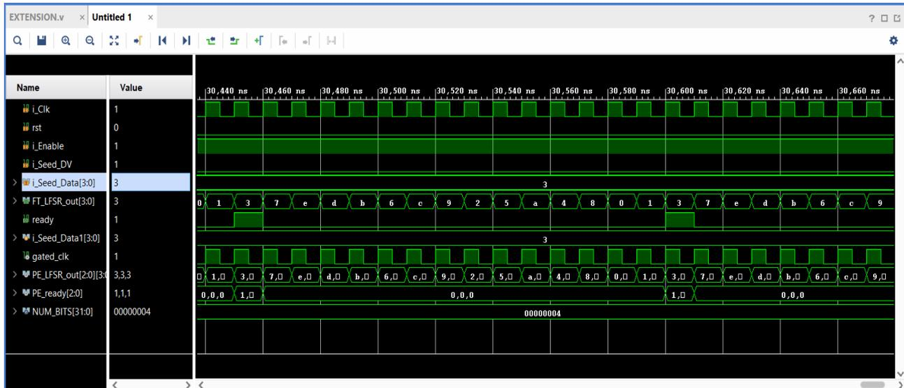
Fig. 5. Simulation Waveform for Proposed FTLFSR
