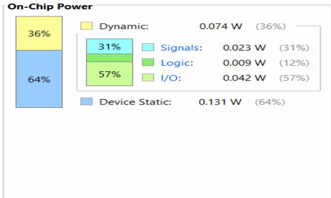
Fig. 8. Power for Proposed FTLFSR
