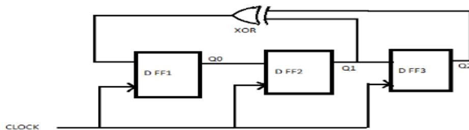
Fig.1: Linear Feedback Shift Register
