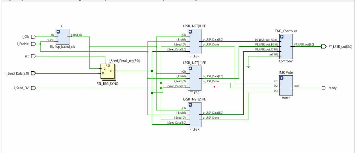
Fig. 4.: RTL Schematic for Proposed FTLFSR
