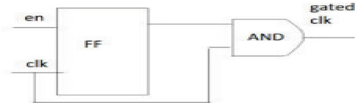
Fig. 3. FLIPFLOP\_BASED CLOCKGATING
