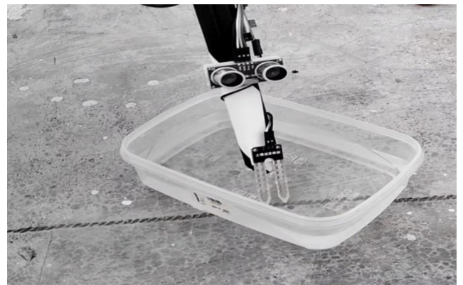
Fig 9: Ultra-sonic and Moisture Sensors
