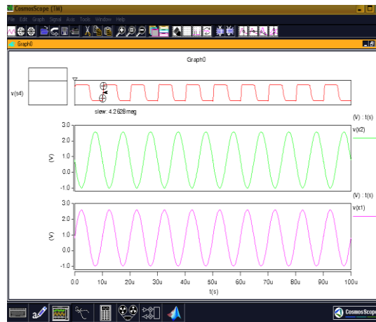
Fig 3(b).Output waveform of push pulls op-amp with current replication branch
