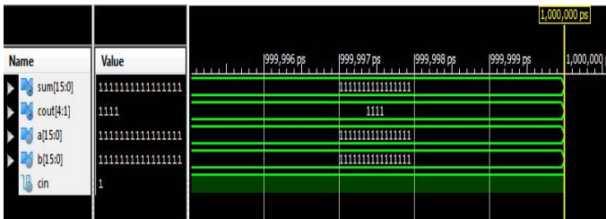
Figure 4.1: 16 bit adder without fast carry logic
