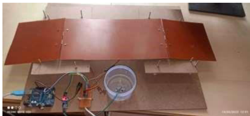
Fig 3: SMART BRIDGE –Top view in Normal Position.
