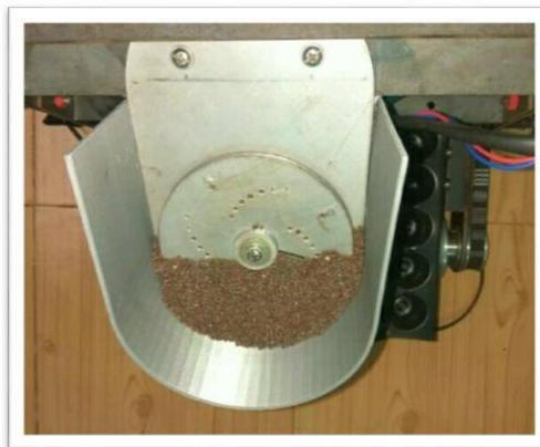
Fig 10: rotor wheel with seeds.
